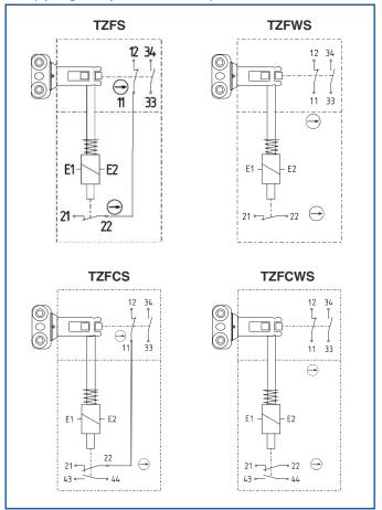
Note: Drawings show contact state with actuator key inserted and solenoid de-energized.
